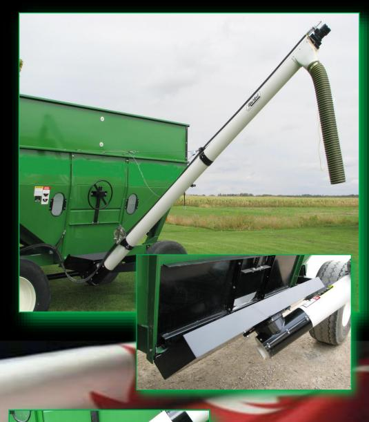
The auger is 2" lower than the door when in transport.
