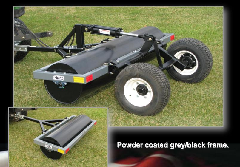
The MARKET HYDRAULIC ROLLER is ideal for all those tight jobs. Available in 4', 5' & 6' widths. The hydraulic lift wheels allow you to move the roller to the job without damage to the surrounding landscape. The heavy duty 16" steel roller is equipped with 2 filler ports for adding and draining water.
