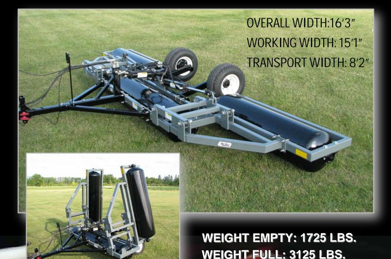
Heavy duty 16" steel rollers are equipped with 2 filler ports for adding and draining water.
