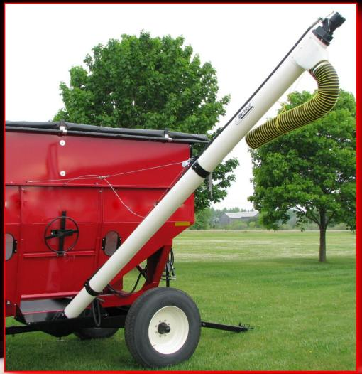
The PIVOT AUGER's design allows the spout to remain pointing downward as the auger is
