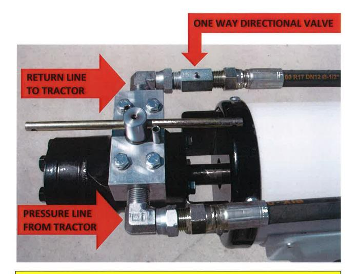
THE ONE WAY DIRECTIONAL VALVE RESTRICTS THE AUGER FROM RUNNING IN THE REVERSE DIRECTION.
