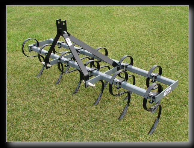
The MARKET COMPACT CULTIVATOR is a 3 point hitch (Cat. 1) unit that performs a multitude of in-field tasks such as seedbed preparation, soil aeration and weed control. Cultivators are available in 4', 5', 6' & 7' widths.
